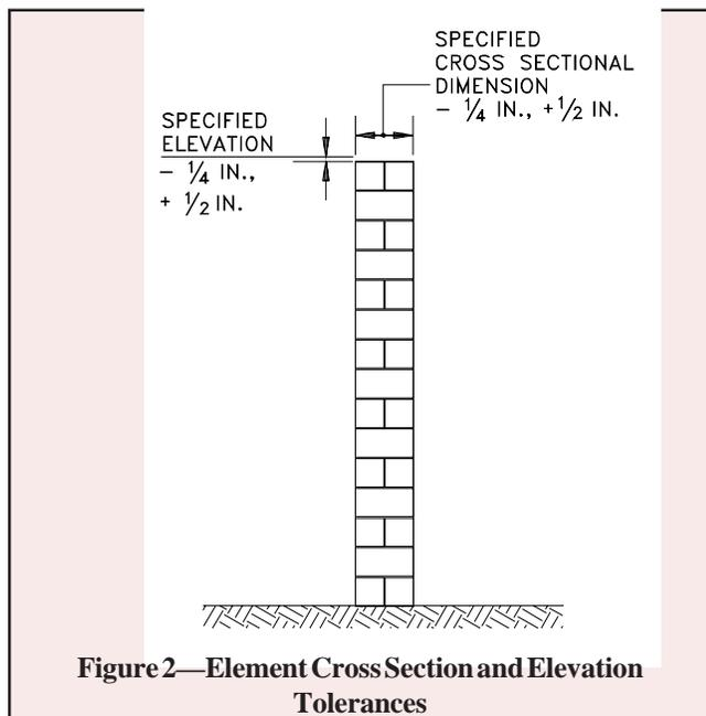
Figure 2—Element Cross Section and Elevation Tolerances
