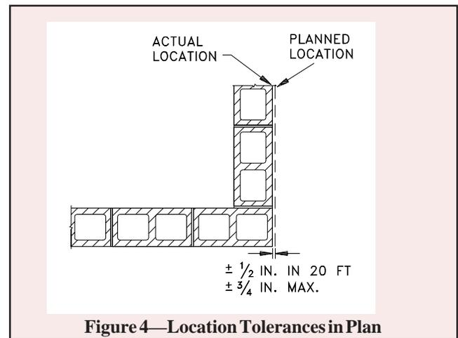
Figure 4—Location Tolerances in Plan
