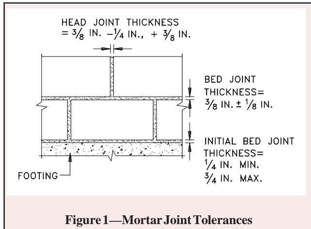
Figure 1—Mortar Joint Tolerances
