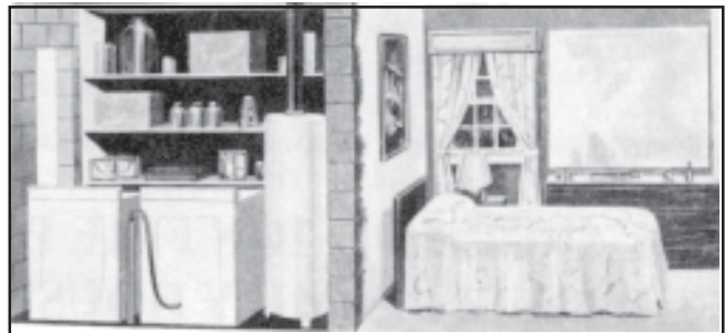
Figure 1—Compartmentation Provided by Masonry Walls Contains a Fire until Brought under Control
