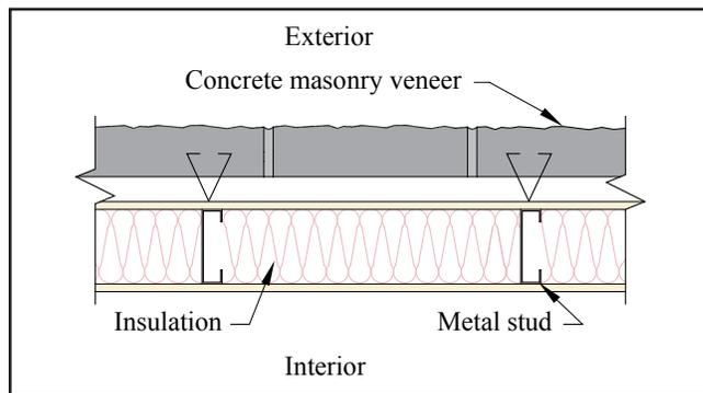
**Figure 2—Concrete Masonry Veneer with Steel Stud Backup**
