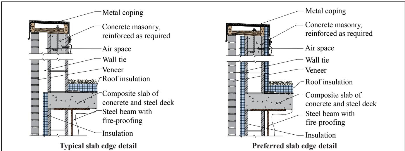
**Figure 4—Alternative Insulation Strategies for a Masonry Parapet**
