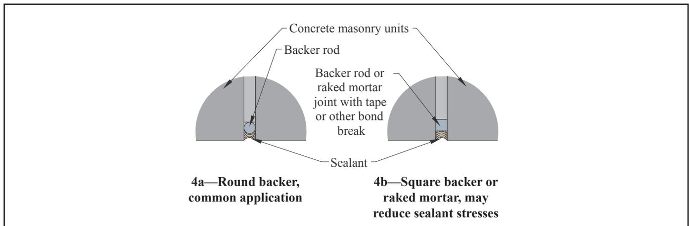
**Figure 4—Detail of Control Joint Surface (ref. 6)**
