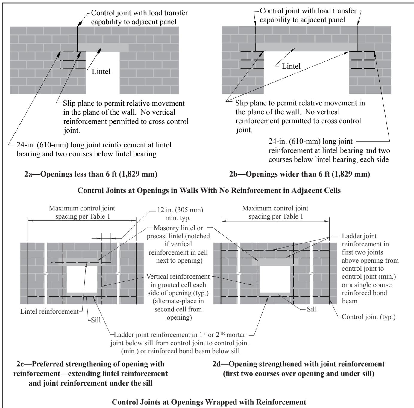
**Figure 2—Control Joints at Openings**
