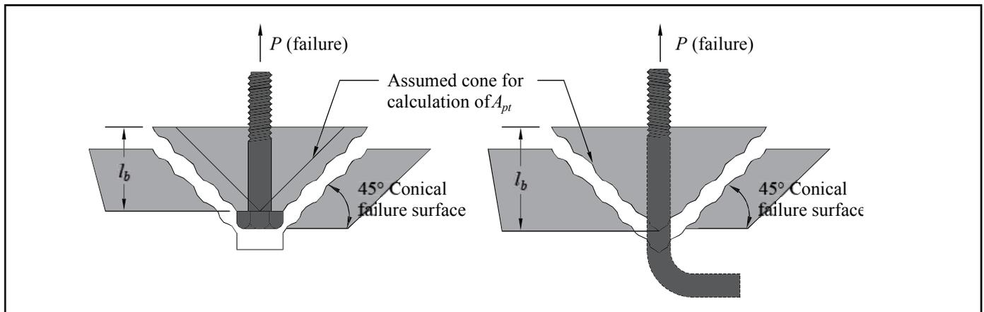
**Figure 4—Assumed Anchor Bolt Failure Cone**
