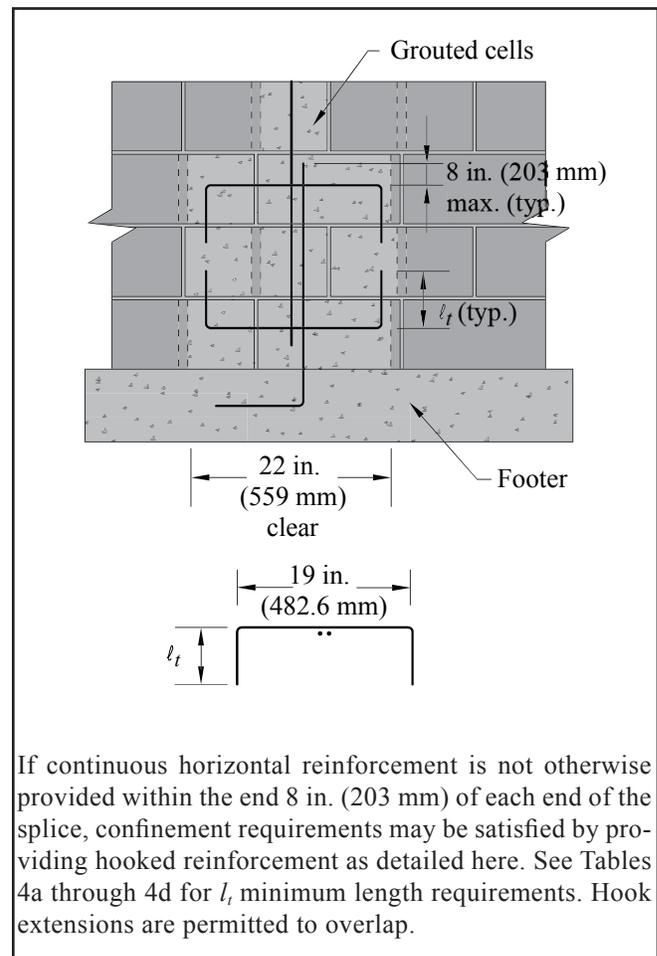
If continuous horizontal reinforcement is not otherwise provided within the end 8 in. (203 mm) of each end of the splice, confinement requirements may be satisfied by providing hooked reinforcement as detailed here. See Tables 4a through 4d for  $l_t$  minimum length requirements. Hook extensions are permitted to overlap.
