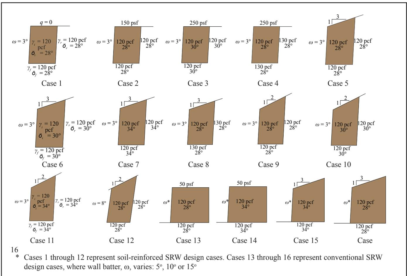
**Figure 1—Design Cases Corresponding to Table 1 and Figures 3 through 5**
