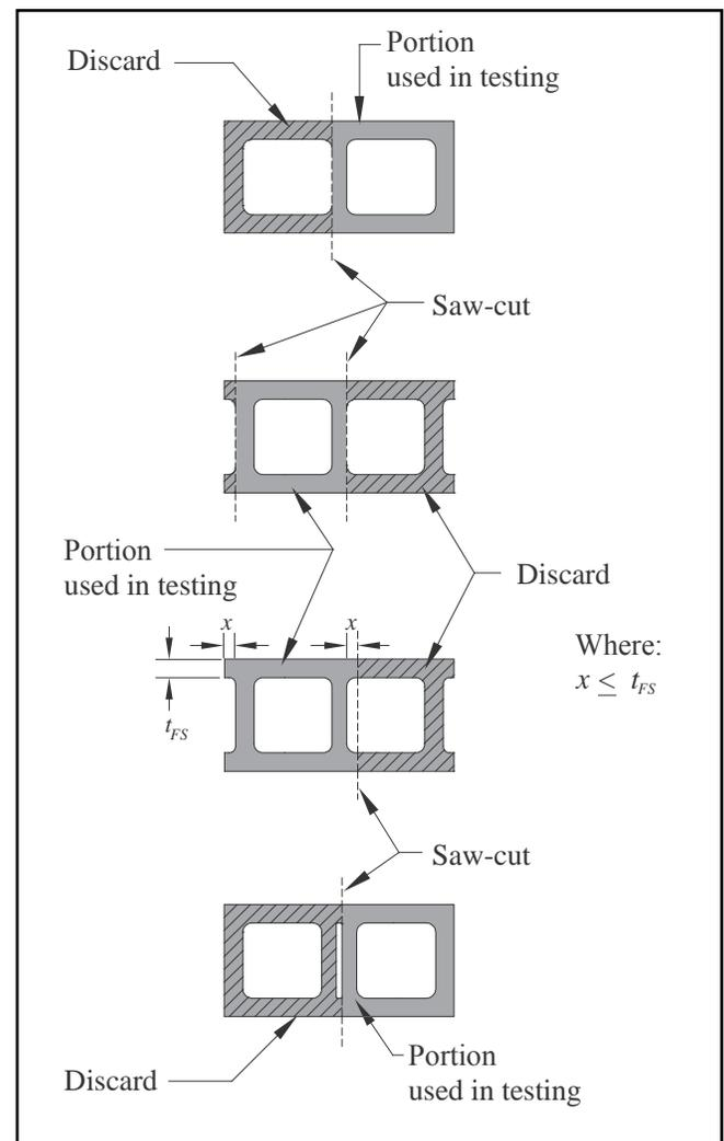
**Figure 2—Saw-Cut Locations for Reduced-Size Prisms**
