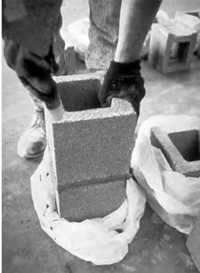
**Figure 3—Constructing a Half-Length Prism in a Plastic Bag**
