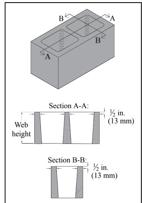
**Figure 1—Measurement of Web & Face Shell Thickness**
