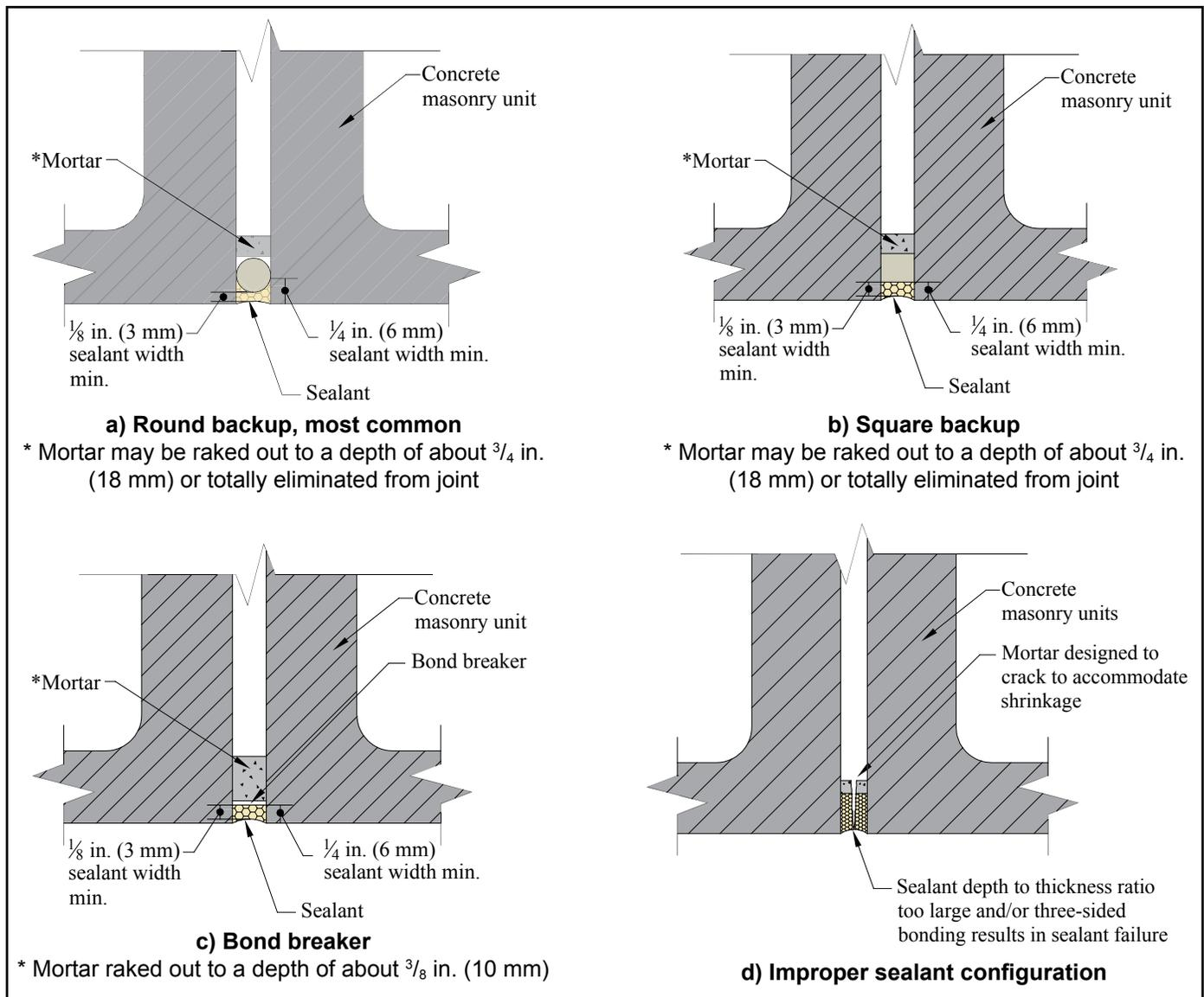
Figure 1—Common Sealant Configurations
