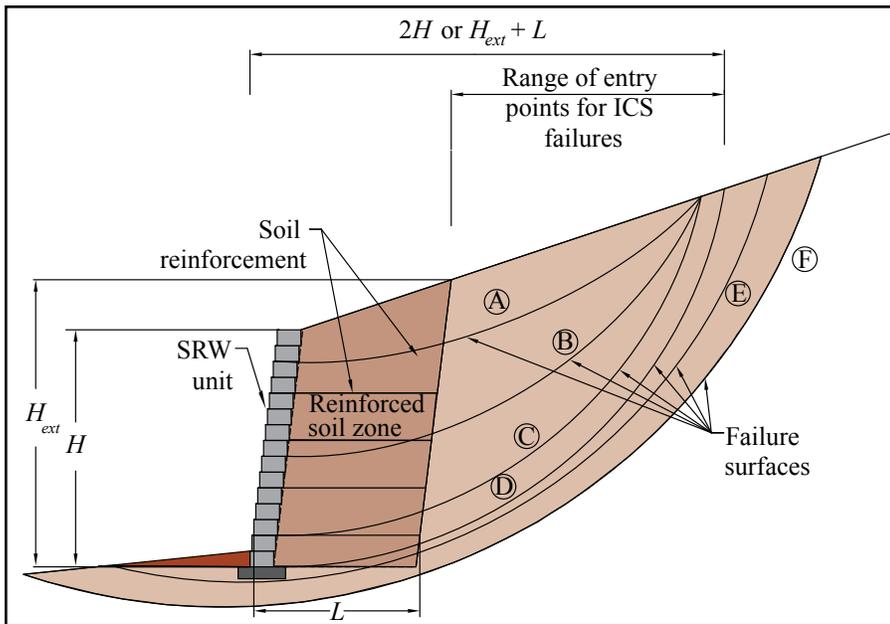
Figure 18. Global Stability Failure Surfaces (Ref. 25)
