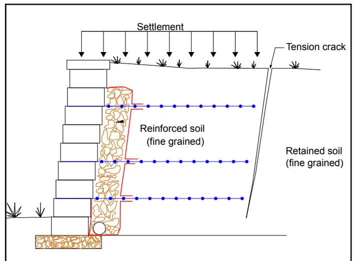
**Figure 7. Failure Due to Poor Compaction behind the Reinforcement**
