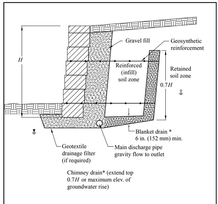
Figure 4. Chimney Drain Example (Ref. 13)
