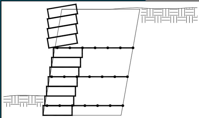
Figure 11. SRW Failed Because the Upper Layer of Geogrid is Missing
