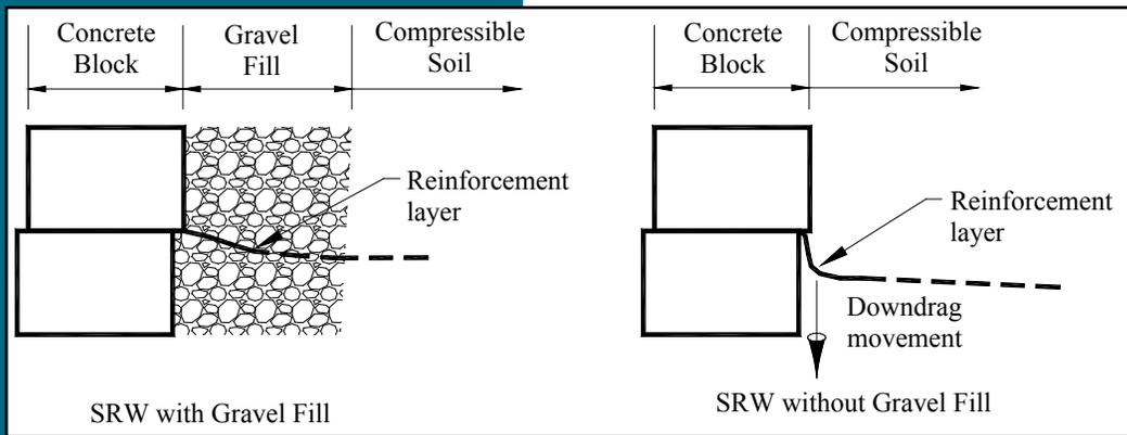
Figure 8. Drag-down on SRW Reinforced Walls
