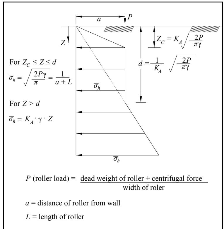
**Figure 9. Compaction Stresses (Ref. 16)**
