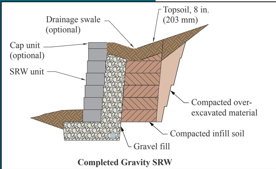
Figure 5. Drainage Swale Used for Surface Drainage (Ref. 9)
