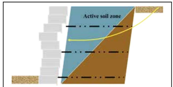
Figure 20. Internal Compound Stability Failure
