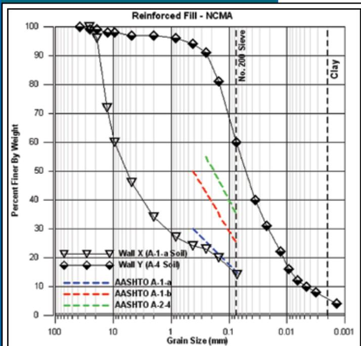
Figure 10. NCMA Test Wall Graduations (Geocomp 2009, Ref. 15)
